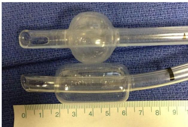
**Fig. 1** Comparison of cuff dimensions of a high-volume low-pressure ETT (*bottom*) and a high-pressure low-volume ETT (*top*). Both ETTs are size 7. The ruler is in centimeters
